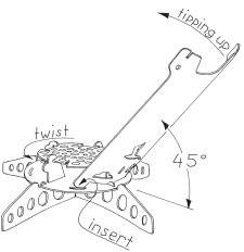
side wall tabs in to grab their metal slot. The process is repeated until all four wall segments are standing. Then put the pan supports into the slots in the side walls. Now our FIBI-Stove is ready for use.
